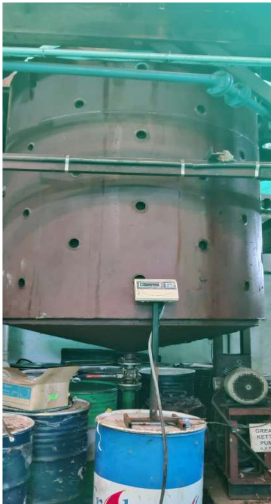
Picture 4: Scrapper Kettle (Finishing Vessel) with bottom filter
