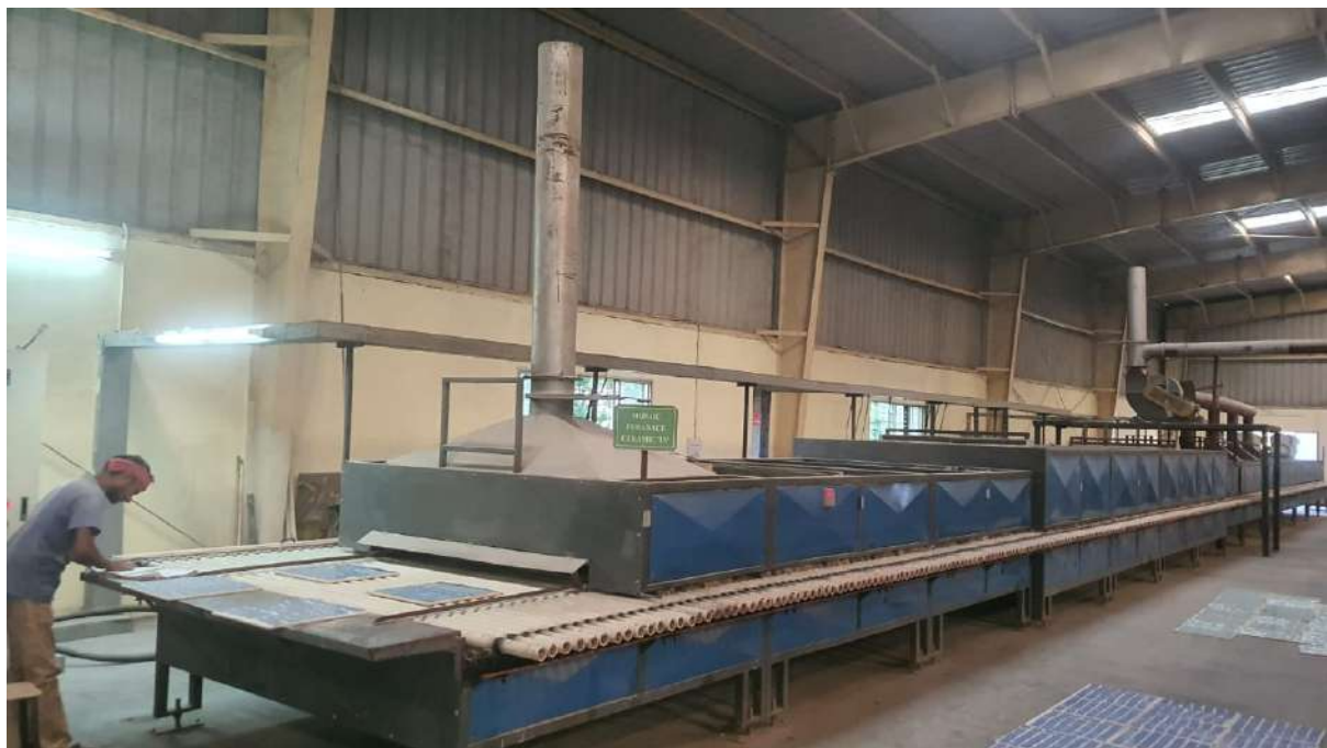
Picture 6: Tiles fed to furnace for preheating and heating
